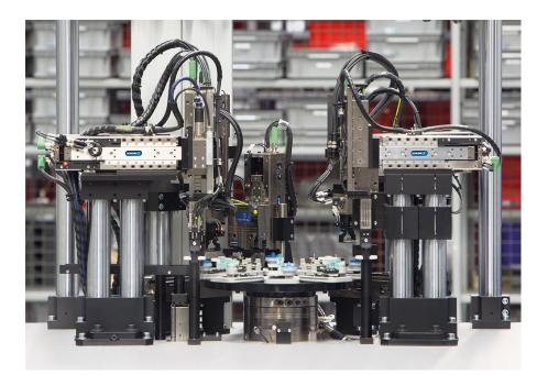
SCHUNK ELP linear axes, SCHUNK EGS rotary gripping modules, and SCHUNK EGP grippers can be combined with efficient 24 V assembly systems. Customers benefit from 24 V technology with minimum commissioning and low maintenance costs, high energy efficiency, and low life cycle costs.
