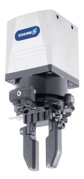
The world's most compact electrical rotary gripper module SCHUNK EGS is available in sizes 25 and 40 with gripping forces of 15 N or 140 N and strokes of 3 mm or 6 mm for component weights up to 0.55 kg.
