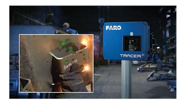
which can be costly and cumbersome. To increase efficiency and reduce scrap/rework, forwardlooking manufacturers have turned toward Laser Projection for templating in applications such as assembly, composites layup, welding, verification, and paint templating.
