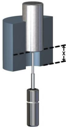
Sometimes, it's not possible to measure the part in a relaxed state. In that case, a probe can be used solely to measure deflection of the part, and the press can be programmed to compensate for that distance.
