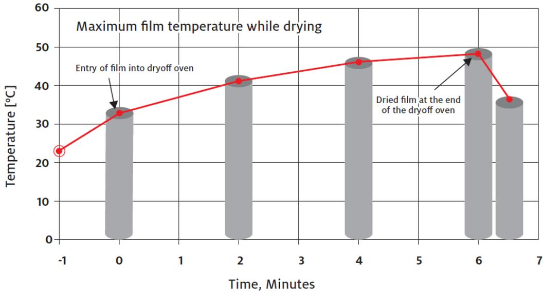
If reactivation will follow immediately, higher drying temperatures can be used to shorten the drying cycle, as exhibited in figure 3.
